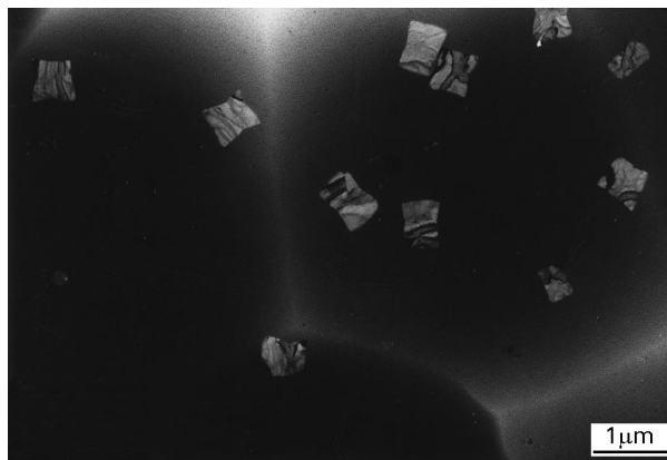
Figure 1 Bright-field transmission electron micrograph of 100 nm thick \text{Ta}_2\text{O}_5 film annealed for 24 h at 600 °C. The film is primarily amorphous with some square to slightly rectangular crystallites.
